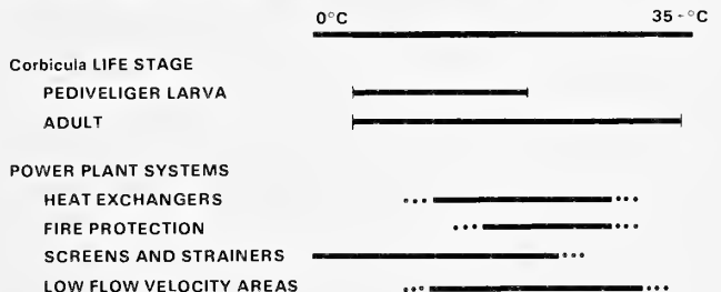
Fig. 4. Categorical model illustrating correlation between temperature tolerances of Corbicula and water temperatures in power plant service water systems.
